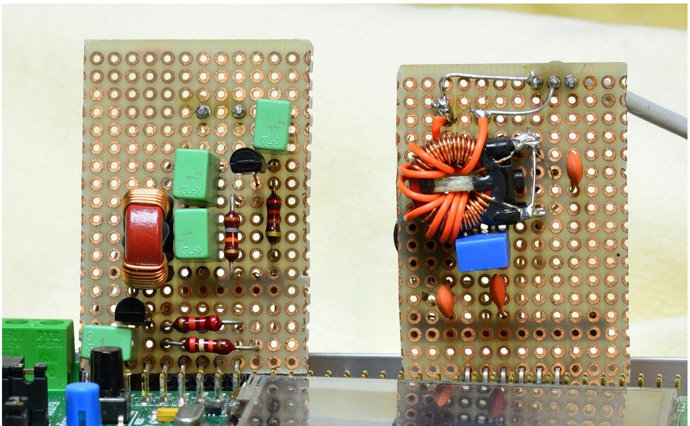
Note : the photo of the right board, that with the input anti alias filter, is of the initial version, that did not have the preamplifier, which was added at a later time
