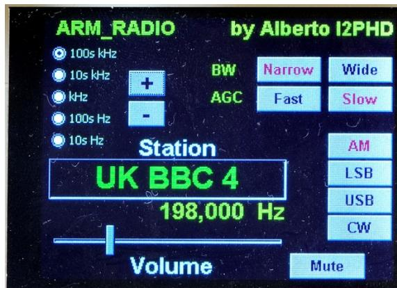
By touching the on-screen buttons, it is possible to change the tuned frequency ( + or - ) by the amount selected with the radio buttons. Also the bandwidth, the AGC speed, the demodulation mode and the volume are all settable with the touch-enabled buttons.
