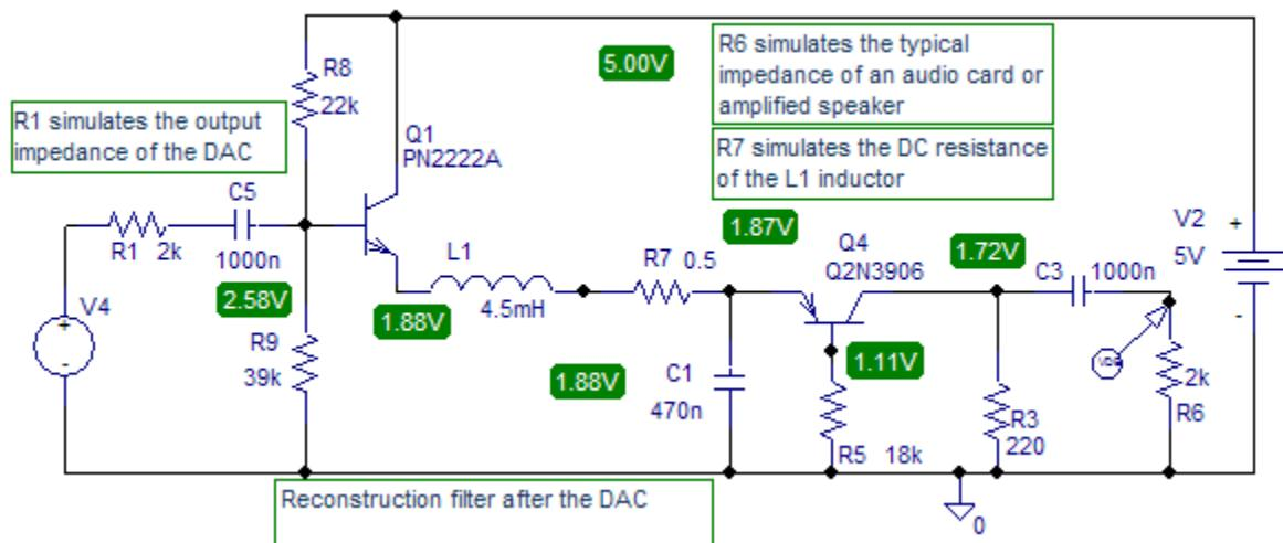
In the actual circuit C5 is connected to bit 5 of GPIOA, which is the output of channel 2 of the DAC.
